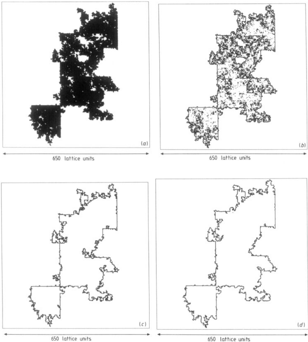
Figure 1. A cluster of 85 870 sites grown using model II. In this model the generator is given by P_1 = 1 , P_2 = 0.1 , P_3 = 0.1 and P_4 = 0.01 ( R_2 = 0.1 ). (a) shows all the 85 870 occupied sites, (b) shows the 17 218 sites in the unoccupied perimeter, (c) shows the 8874 external hull sites and (d) shows the 5658 internal hull sites.
